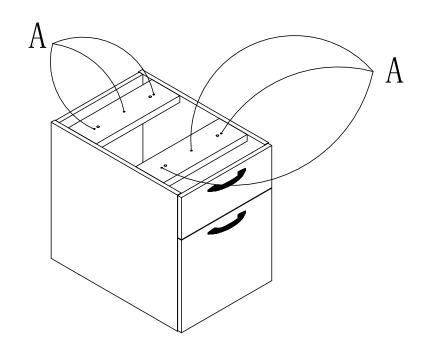
If the underside of the worksurface panel is larger than 25mm as shown in figure A, Please use the 6 provided WOOD SCREWS to attach the pedestal. Secure the Pedestal by the 6 smaller Screw holes in the Pedestal.
