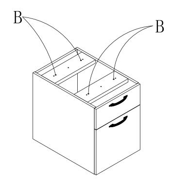
If the underside of the worksurface panel has BOLT HOLES as shown in figure B, Please use the 4 provided BOLTS & WASHERS to attach the pedestal to the panel. Secure the Pedestal by the 4 Larger BOLT holes in the Pedestal.
